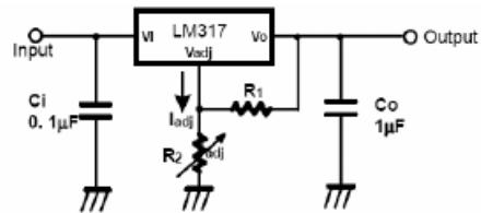
$$V_o = 1.25V \left(1 + R_2/R_1\right) + I_{adj}R_2$$
