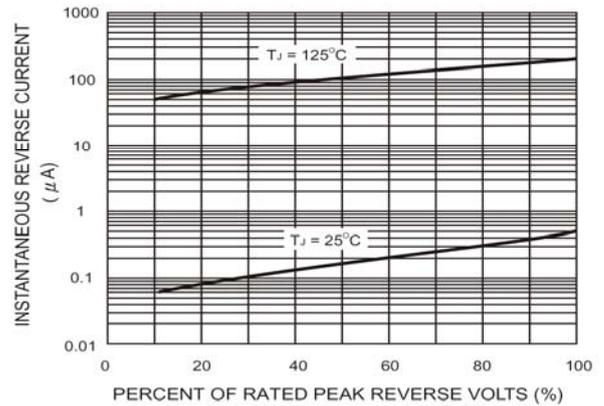
Figure 4. Typical Reverse Leakage Characteristics Per Bridge Element
